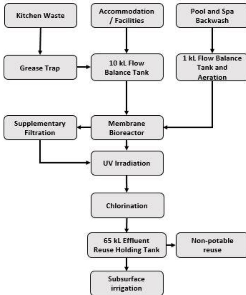
Figure 1: Wastewater management scheme configuration.
