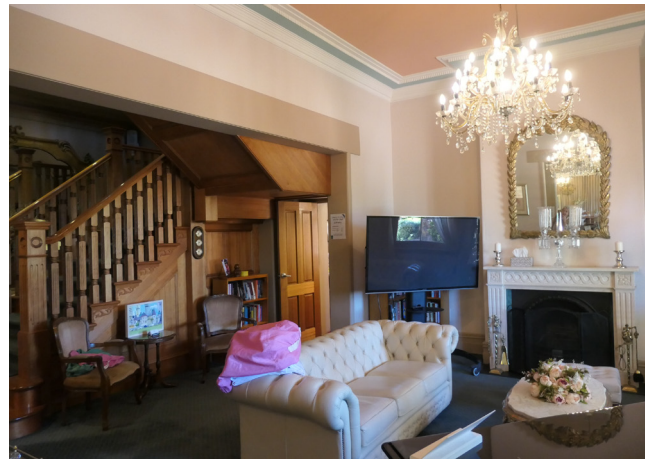
Figure 3.10 Ground floor interior of Collaroy House. The fireplace and corning may be original but the wide opening and staircase are later alterations.
