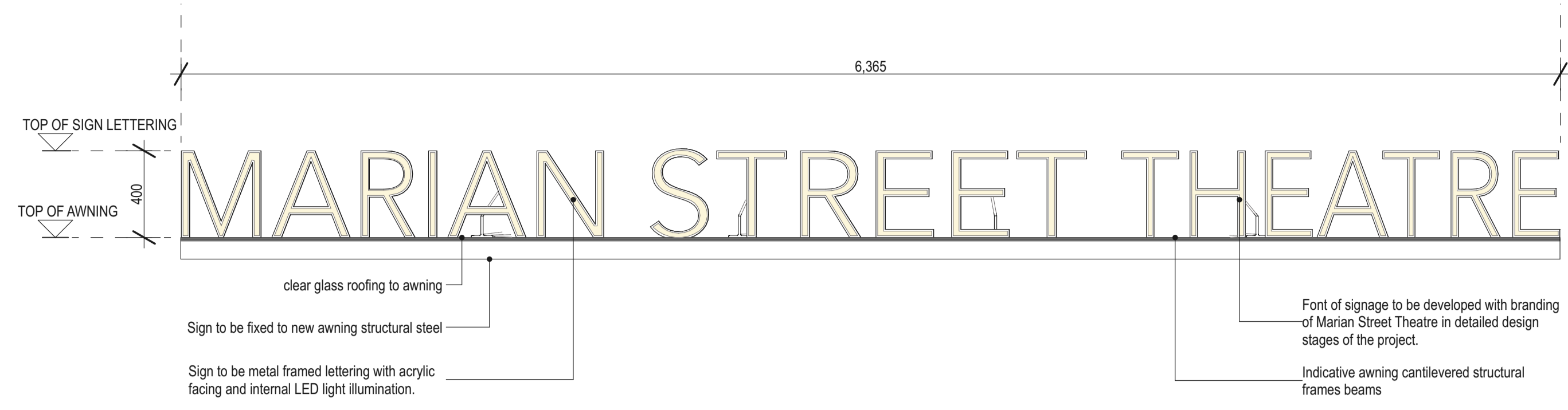
2 SIGN 01 - ILLUMINATED AWNING SIGNAGE ELEVATION 1:20
