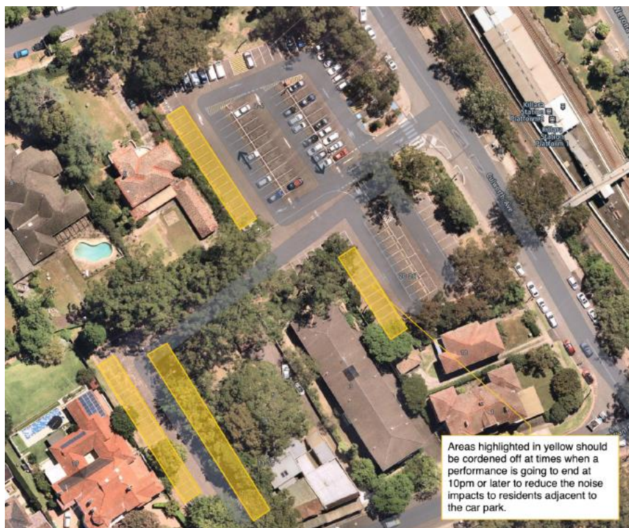
Figure 3 Acoustically constrained spaces (shown in yellow)
