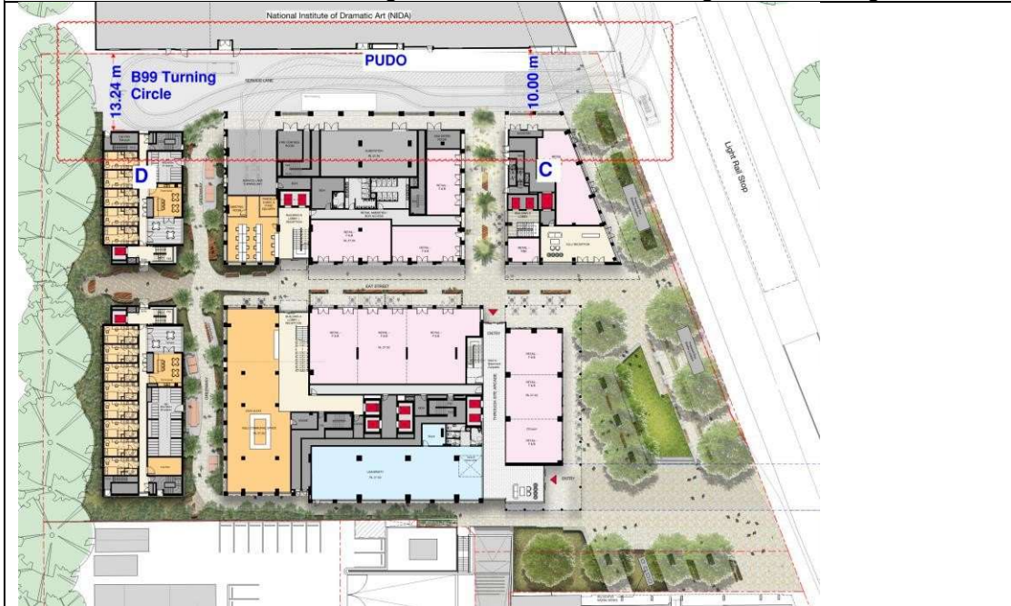
Figure 1: Shows the increased setbacks of Building C 10m from the north including 3m wide colonnade and building D setback 13.4m enabling a B99 turning circle.
