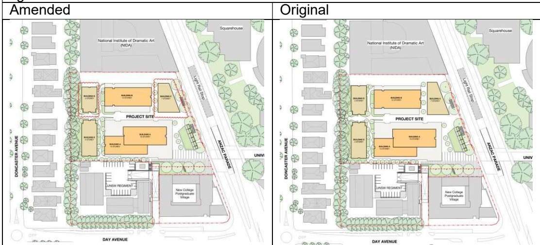
Figure 2: Proposed site plan as amended showing layout changes clouded red being building D and C shifted further south and increased northern easement -see also figure 3 and 4 further below.
