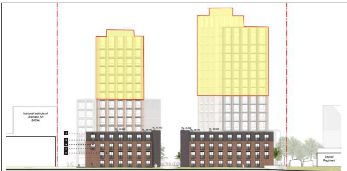
Figure 35: Western elevation showing the variance in size and scale between the proposed and a compliant scheme.
