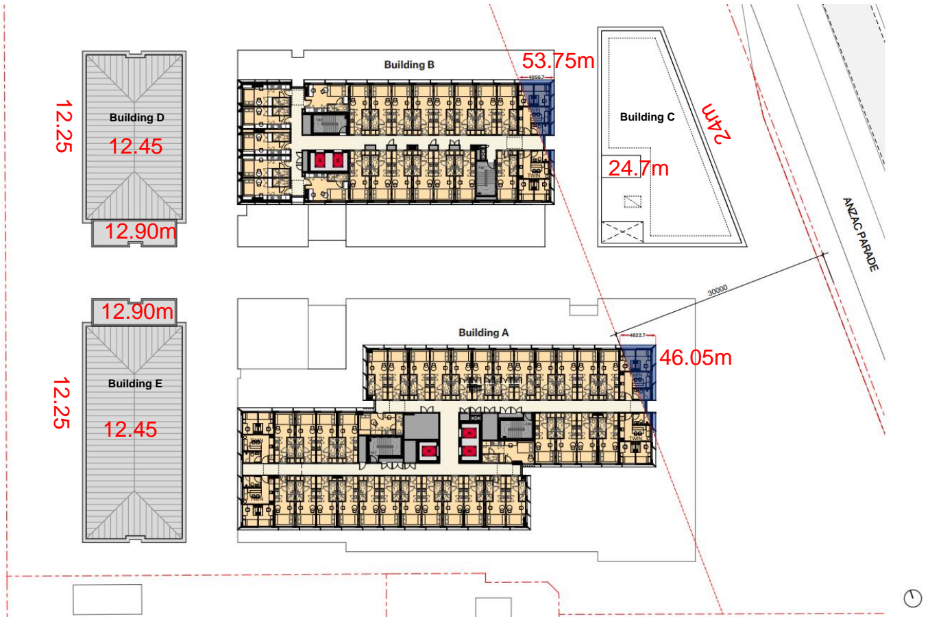
Figure 4 Proposed Site Plan (extent of proposed variation in blue) indicating extent of encroachment into 24m height zone in blue
