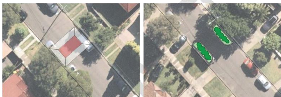
Left to Right: Flat top road hump, road narrowing (kerb blisters with landscaping)
