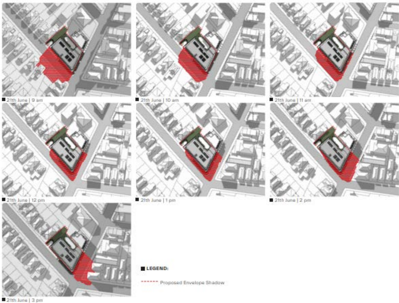
Figure 5 | Envelope shadows of proposal between 9am and 3pm on 21 June (Source: Urban Design Study)
