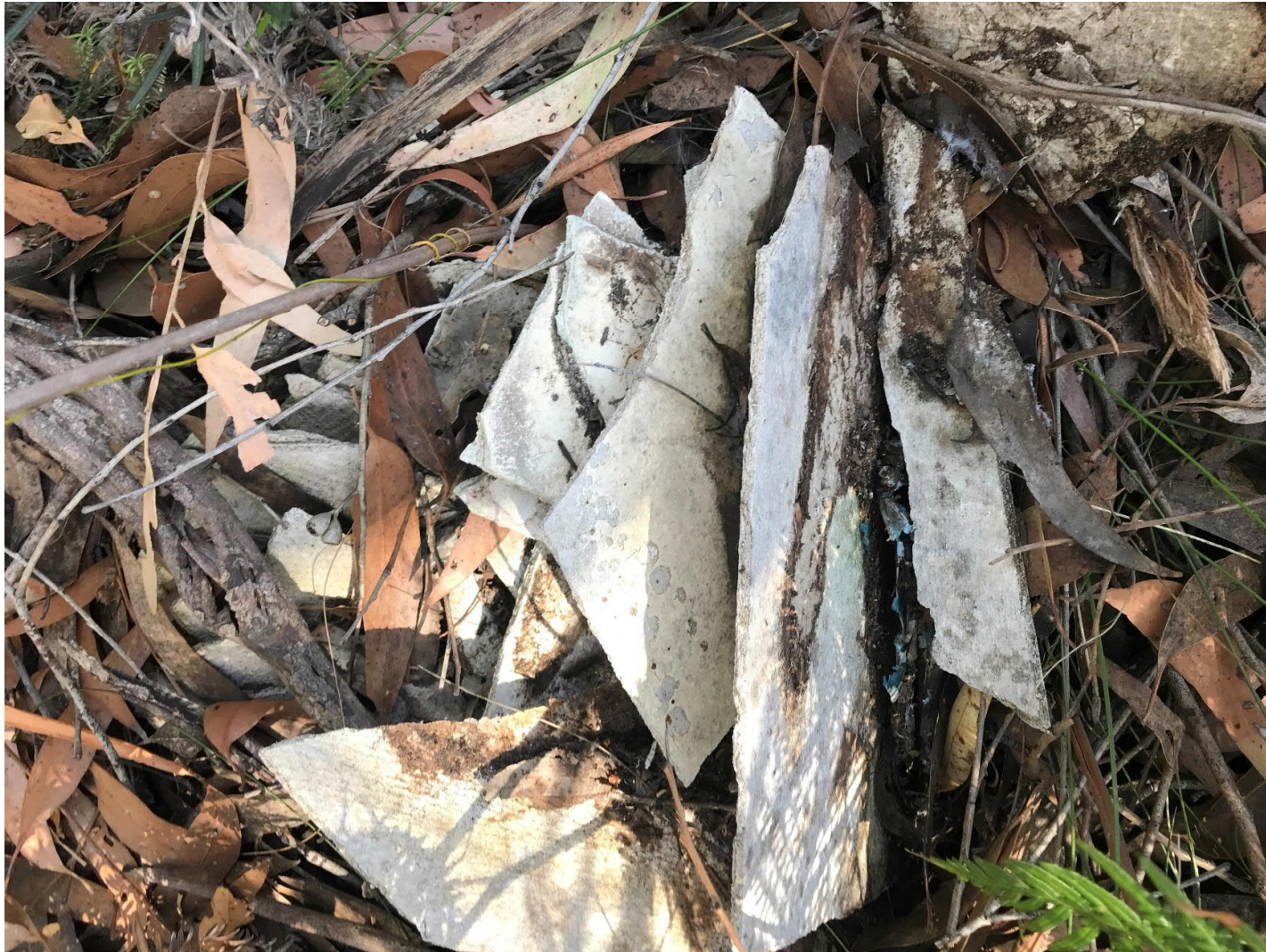
Photograph 6: Asbestos cement sheeting in semi buried condition
