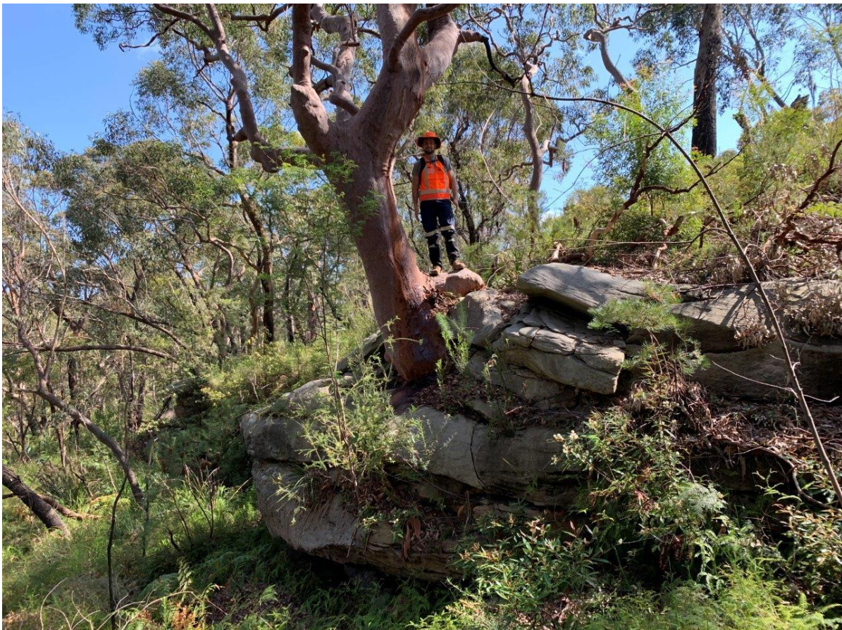
Photograph 16: View looking north, mature tree at crest, loose undercut blocks at crest
