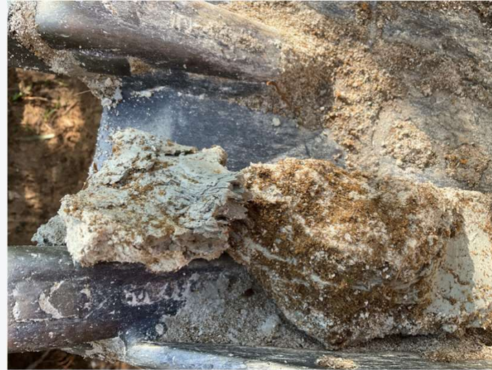
Photo 6: 29/06/2022 Example of spoil material from test pit TP01.
