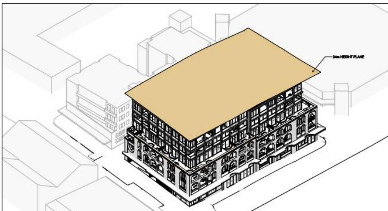
Figure 7: 24m height plane (source: SJB, December 2022)
