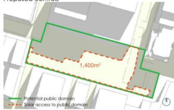
Figure 38 - 1,300m² of sunlight in existing and new public domain areas at Grosvenor Lane under proposed controls on 21 June at 10am
