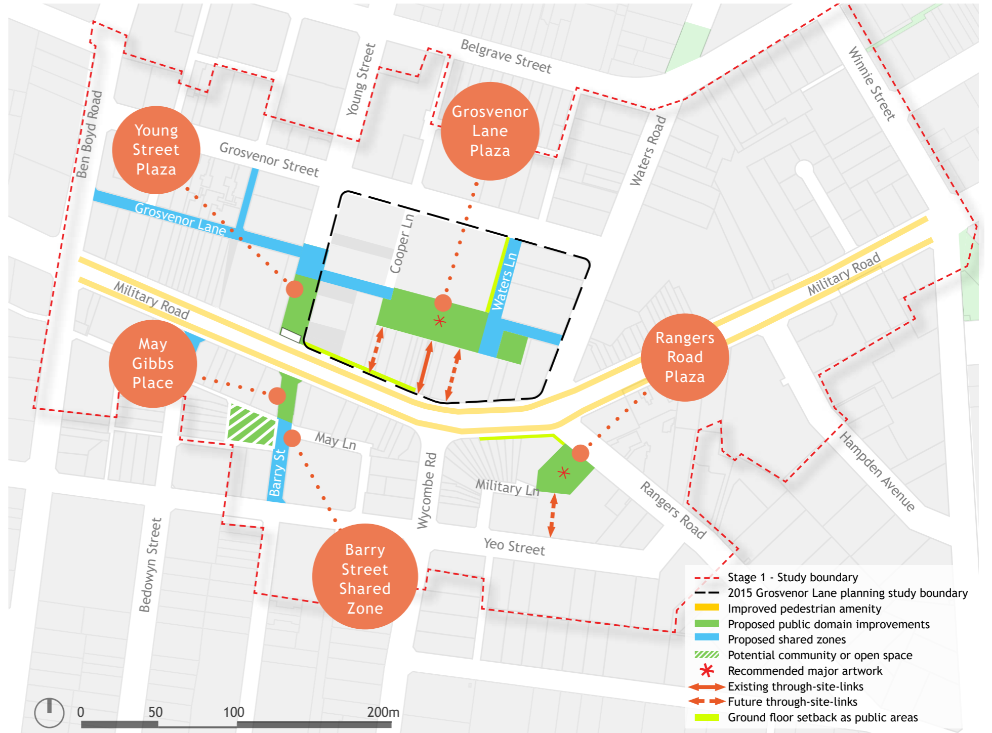
Proposed public domain strategy for Netural Bay town centre focusing on pedestrian and public domain improvements throughout the town centre including the provision of new open space (Ref: North Sydney's 'Military Road Corridor Planning Study Stage 1')
