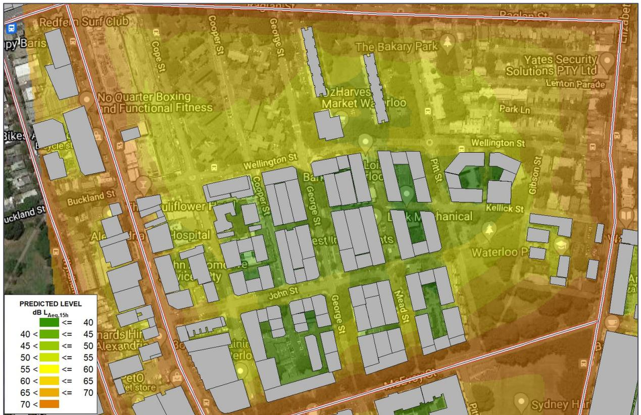
Road traffic noise levels from McEvoy Street are in the order of 65-70 dB L<sub>Aeq,15hr</sub> at the building facade closest to the road. These levels will trigger the need for acoustic upgrades to these façades. The noise impacts reduce as the receiver location moves further into the site. Dwellings within 80 m of McEvoy Street will need to be assessed at development stage to determine required facade acoustic performance and the need for alternative ventilation.
