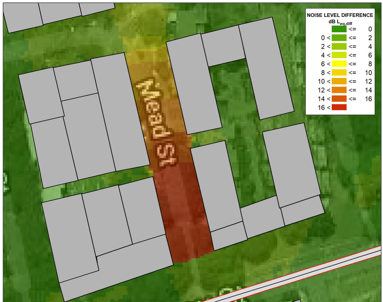
Noise levels external the buildings (east/west facades) fronting Mead Street may therefore be at a level where windows to bedrooms would need to be closed to achieve relevant internal noise levels and/or additional sound insulation treatment would likely be required. With a requirement for windows to be closed, there is likely the need to provide mechanical ventilation.
