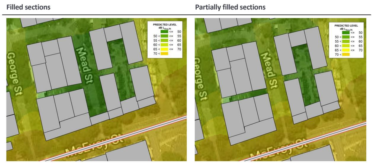
Figure 7 shows the relative change in road traffic noise levels for the two (2) schemes. With the partially filled arrangement, road traffic noise levels are expected to be more than 10 dB higher at the respective facades of buildings (east/west) fronting Mead Street.
