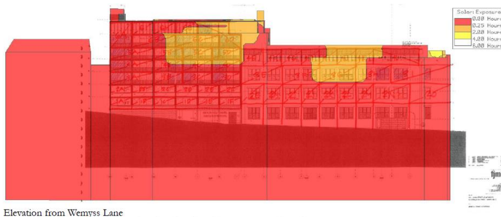
Figure 11: Western elevation of Meta building to Wemyss Lane, showing solar impacts of proposed planning envelope at northern end of street block (4-22 Wentworth Ave) and southern end of street block (24-44 Wentworth Ave). Red indicates 0-0.25 hours, orange indicates 0.25-2 hours and yellow indicates 2 hours plus
