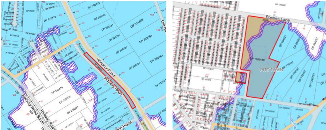
Figure 8 Site 1 – Vineyard (L) and Site 2 – Pitt Town (R) 1 in 100 year flood mapping
