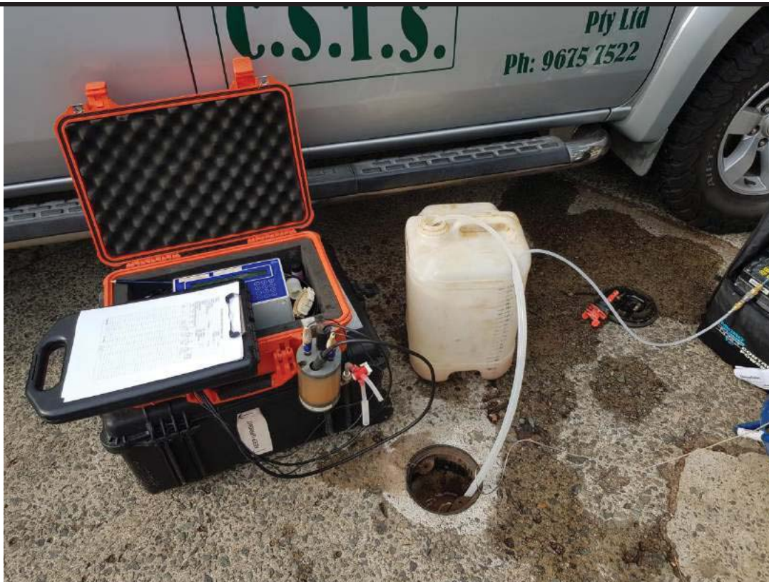
I: Groundwater Sampling Equipment in MW3
