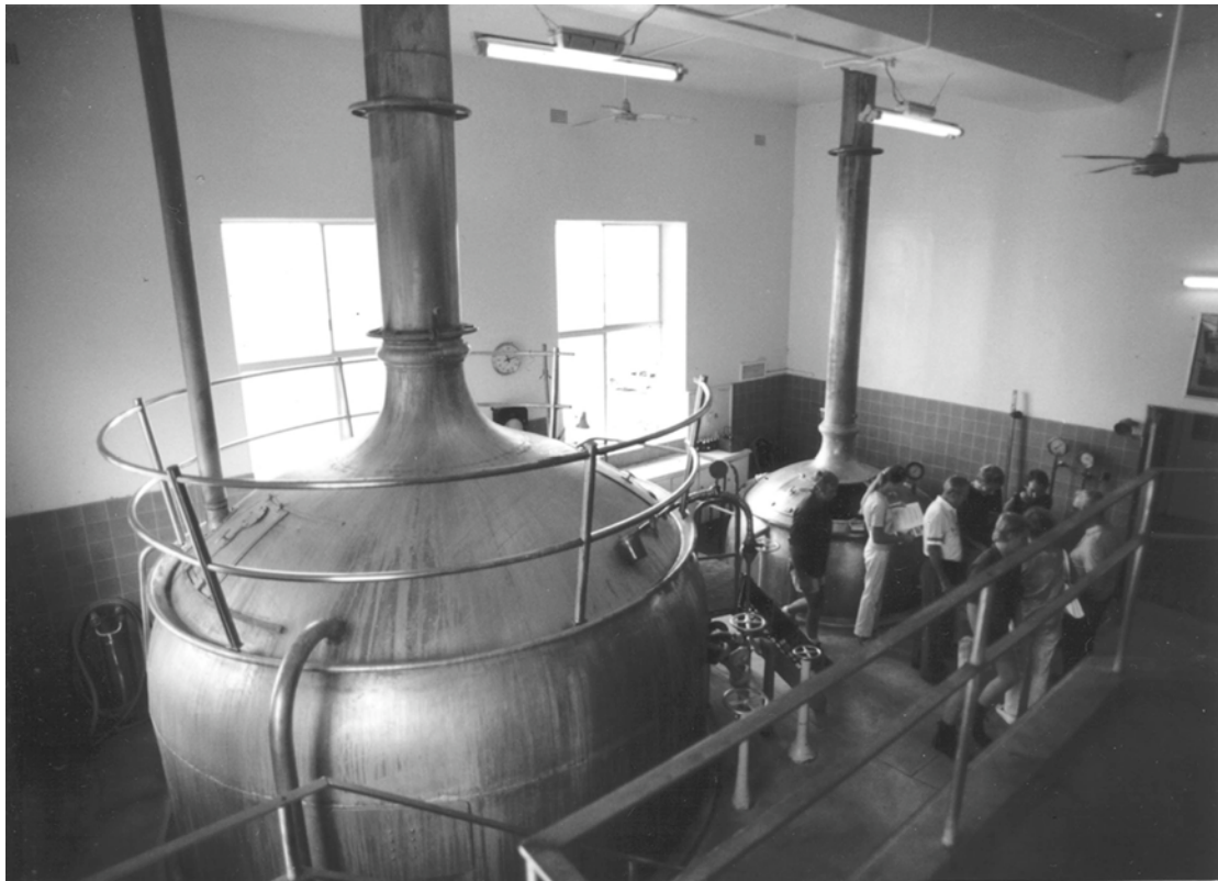
Figure 4.3 The brewhouse at the Grafton Brewery, 1988. These copper brewing vessels were manufactured by A. Ziemann Breweries of Ludwigsburg, near Stuttgart, Germany. As far as can be ascertained, they were scrapped soon after the closure of the brewery.
