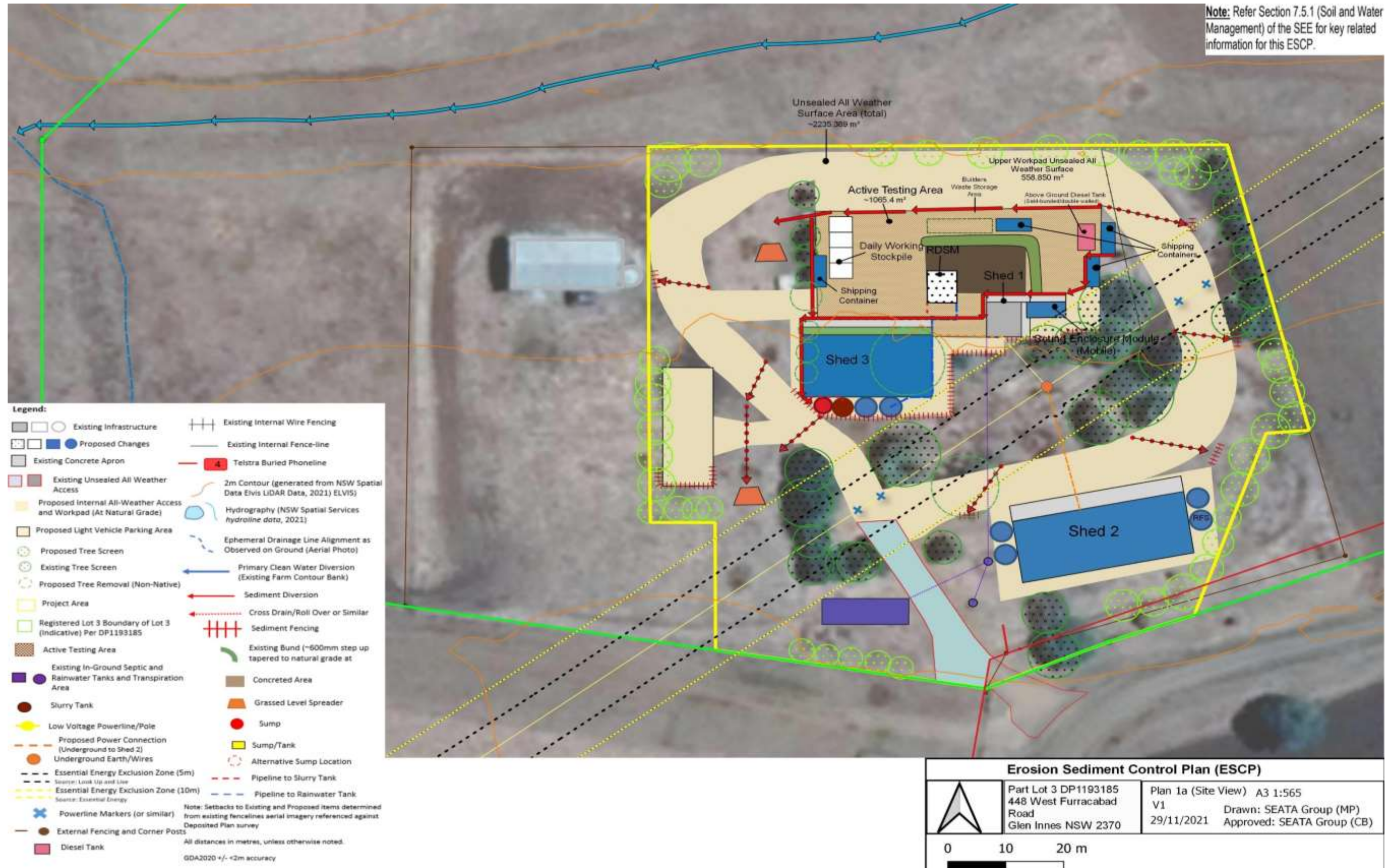
Figure 2.2. ESCP for the SEATA R&D Centre at Glen Innes, NSW. The sediment sump drained from the Active Testing Area will be tested to ensure suitable for conventional management as expected, or otherwise transferred to the adjacent slurry tank for disposal.
