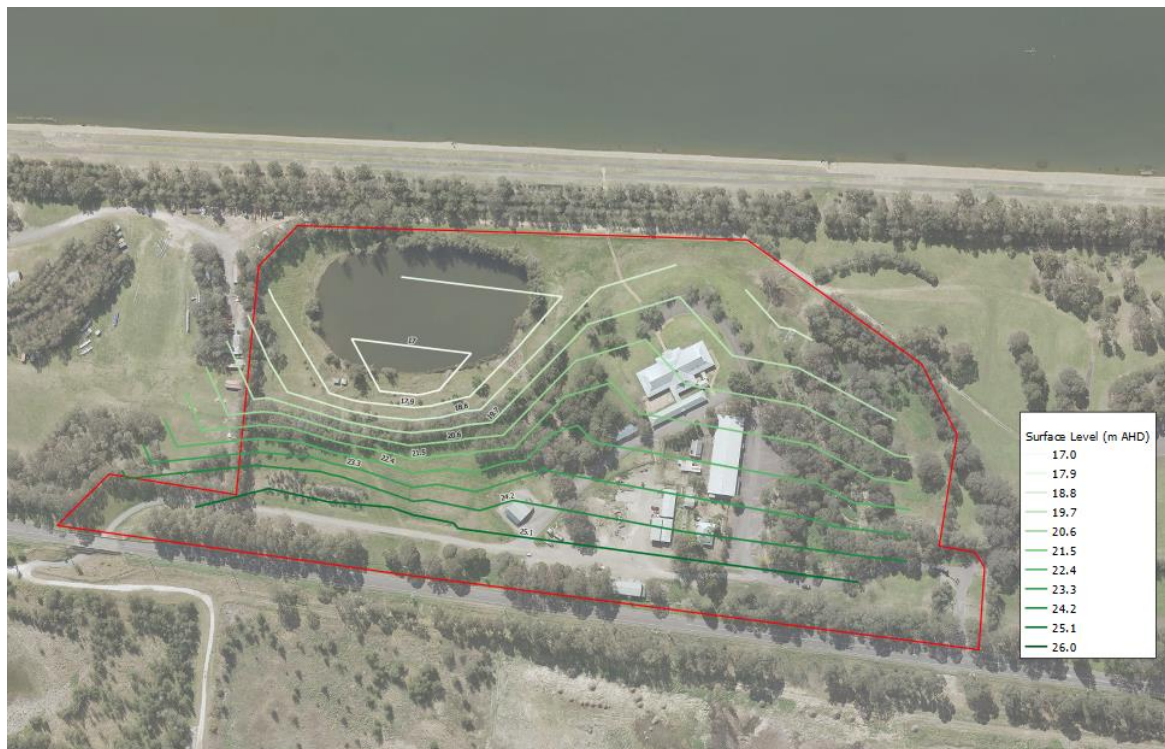
Figure 3: Site Topography (surface levels obtained using dGPS)
