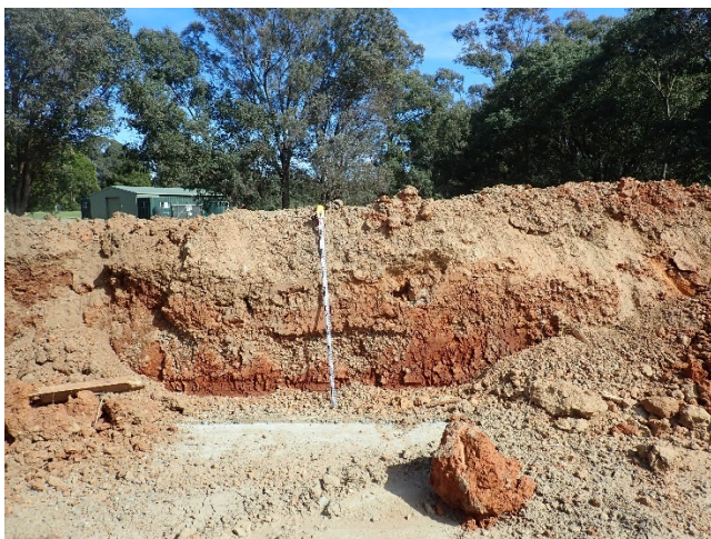
Figure 14 – Exposed redeposited clay north-west of single storey cottage
